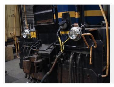
Designed for application to yard switcher locomotives without necessary ditch lights per TC and FRA rules.
